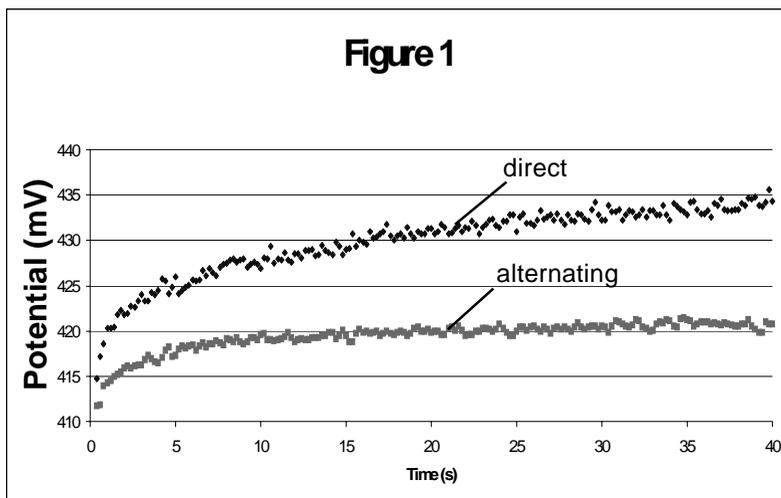
In a conventional system with dc current the electrodes are polarised, and become the site for reactions other than the reaction iodine to iodide. This leads to a drift in the potential difference between the electrodes and an end point that may be erroneous.
